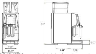
PLEASE NOTE: Power can be installed under or above counter. Please allow 3-4" of space for the plug, especially when placing power above the counter and behind the machine.
