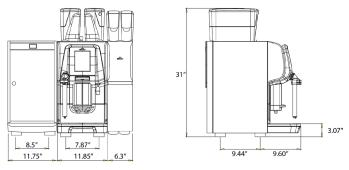
PLEASE NOTE: Power can be installed under or above counter. Please allow 3-4" of space for the plug, especially when placing power above the counter and behind the machine.
