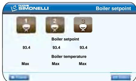
Select the coffee boiler to be adjusted and confirm by pressing the rotary switch.
