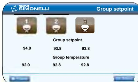
Use the rotary switch to select the coffee boiler for offset adjustment and press it to proceed. Also use the rotary switch to set the offset value for the group and then press the switch to confirm.
