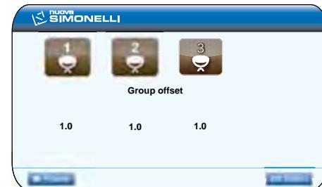
With the rotary switch it is possible to select the group offset to be adjusted and press to proceed.
