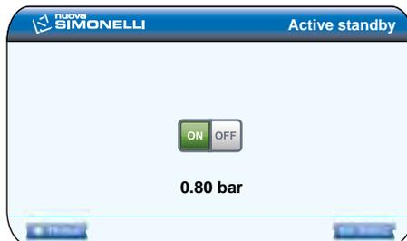
Press the rotary switch to confirm the required option.
