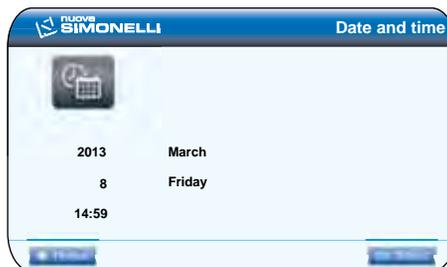
Once the icon has been selected with the rotary switch, press it to access the change mode for the year, month, day, hour and minutes. After the minutes have been set, the machine returns to the main menu.
