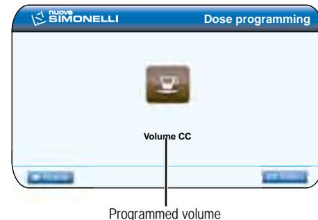
It is possible to change the dose using the rotary switch and then pressing it to confirm the setting. Or, press the coffee key to programme, the delivery will start and in the meantime, all of the other lights will switch off.
