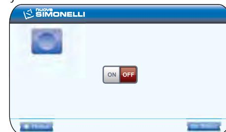
Selecting ACTIVE it is then necessary to use the rotary switch to set the hours and minutes after which the alarm message appears. After the minutes have been set, the machine returns to the main menu.
