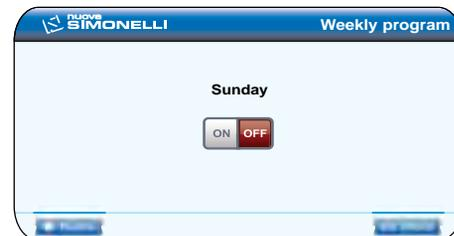
To save changes, press the rotary switch. At this point, the day is active, the hours will start to flash for the ON time.
