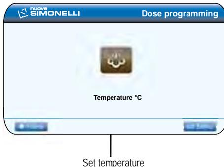
It is possible to change the temperature using the rotary switch and the press to confirm the setting. Or, press the steam key to programme, the delivery will start and in the meantime, all of the other lights will switch off.
