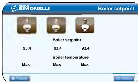
Hold down the washing key to access offset and boiler temperature adjustment.
